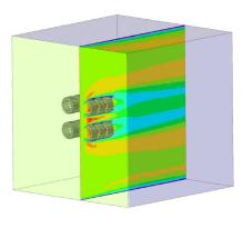
Induction heating simulation capabilities were extended with support for 2D plane strain model symmetry, B-H curves, hysteresis losses, electrical/magnetic field intensities, electrical current density and magnetic flux density.
