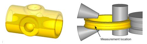
The Ring Rolling template gained support for a user-specified ring diameter measurement location (above; right). The tracked inner or outer diameter is utilized in stopping and movement controls that depend on ring diameter or growth speed. A ring roller PID control was added to support these features.
